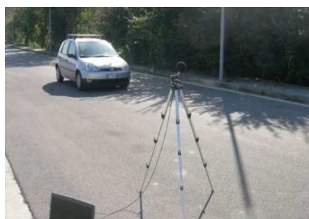
Figure 1 - a) Pass-by di ICEV diesel; b) Livelli massimi medi del pass-by per tipo di veicolo e velocità - a) Pass-by of the diesel ICEV; b) Average max pass-by levels for each type of vehicle and pass-by speed.
